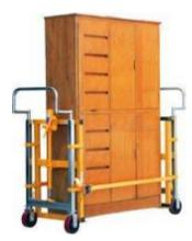
The cabinet being transport must not be left unattended standing on the equipment; it must always be lowered onto the floor.
